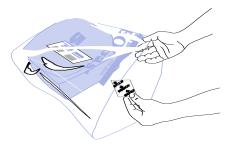
Remove an EOGas cartridge from the dispenser box. Confirm that the number printed on the EOGas cartridge corresponds with the number printed on the sterilization bag. Remove the trigger guard (secured with green tape) and place the EOGas cartridge on top of the devices near the open end of the sterilization bag in a horizontal orientation (long edge of cartridge as parallel to the floor as possible), but **do not activate the cartridge at this time.**
